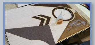
4) Apply a small amount of wood glue to each of the teeth in the joints. Secure in place with wood clamps and allow it dry for 30 - 40 minutes. Once the glue has completely dried, sand and finish.
